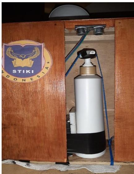
**Gambar 2.** Alat Automatic Hand Sanitizer
